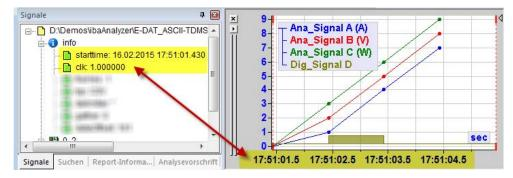
Fig. 4: Representation in ibaAnalyzer with starting time read out and computed timebase.
