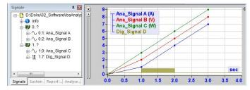
Signals structured in the signal tree. Digital signal "Dig\_Signal D" is displayed like a digital signal.
