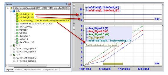
Fig. 7: Display of the Info fields in ibaAnalyzer
