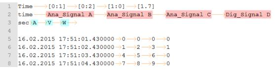
Fig. 5: Signal names (red) and signal units (blue)
