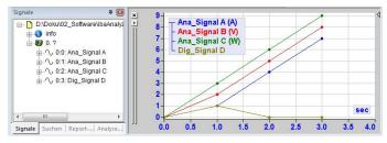
In the signal tree, signals are on one level. The digital signal "Dig\_Signal D" is displayed like an analog signal.
