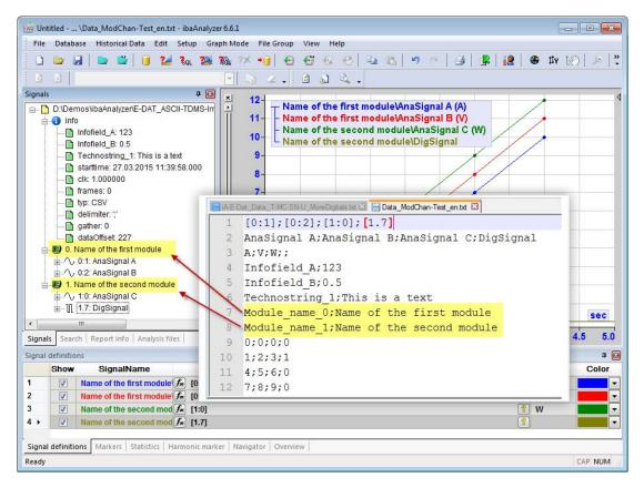
Fig. 8: Definition of module names in the text file and the result in the signal tree of ibaAnalyzer
