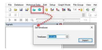
Fig. 13: Prompt for entering a time base when opening a file without time column
